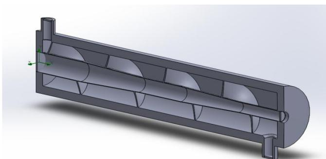
**Figure 1.** Cross sectional view of baffle.
