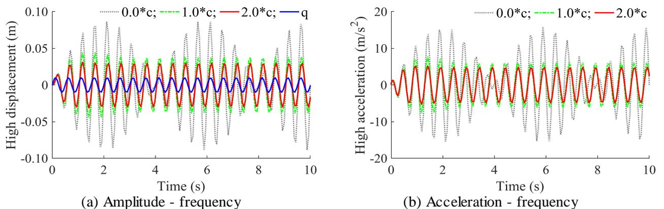
**Figure 3.** The effect of the damping coefficient on the vibration response of the automotive suspension system in the time region.
