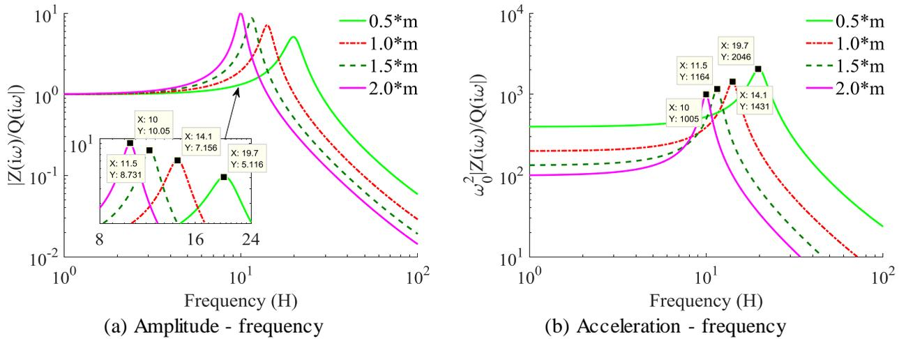
**Figure 5.** The effect of the automotive mass on the vibration response of the automotive suspension system in the frequency region.
