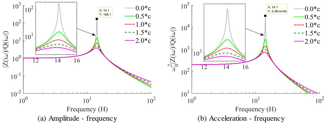
**Figure 2.** The effect of the damping coefficient on the vibration response of the automotive suspension system in the frequency region.
