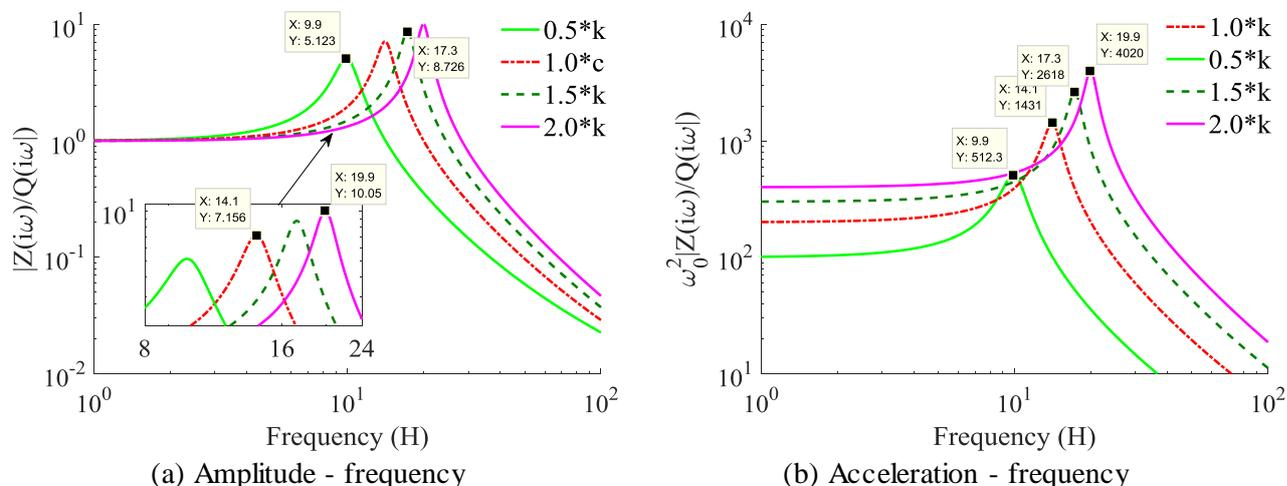
**Figure 4.** The effect of the stiffness coefficient on the vibration response of the automotive suspension system in the frequency region.
