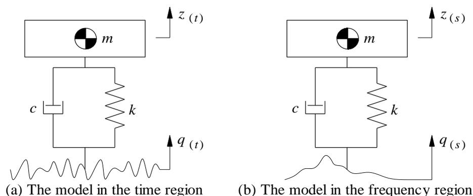
**Figure 1.** The simple dynamic model of the automotive.
